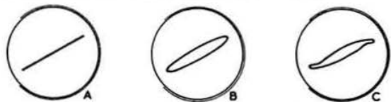
Fig. 2. Patterns produced by applying the input and output of the modulator to the X and Y plates of an oscilloscope. A—No phase shift or distortion; B—Slight phase shift; C—Phase shift and distortion.
